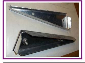
The former holes will be used later to bolt on the elevator balance weights. I'm pleased with the results.
