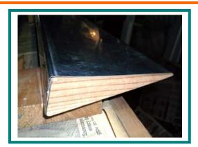
The next step was to use this wood block and trace it onto two pieces of flat, 1/8" steel flat bar, which I then cut out with a hack saw, smoothed the edges and then rounded the edges of one piece so that forming aluminum over it would not stress crack the aluminum. Note the female steel form plate is about 3/32" smaller than the tight fitting wood block.
